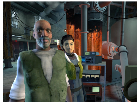
Figure 13: Ambient cubes in action - two characters integrated into a complexly lit scene - from the left white / bluish light strikes the characters, while from the right they are softly lit by red light originating from the liquid in the background. See section 5.
