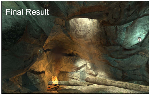
Figure 11: The final result. Additionally to directional lightmapping, the specular part has been computed. In the image the difference is hardly visible; since the specular part is view-dependent, the difference is better visible when the camera moves through the scene. Image taken from [McT04]; see section 4.5.
