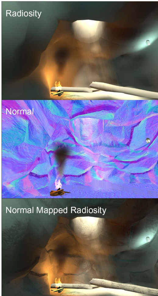
Figure 9: This figure illustrates the combination of lightmaps and a normal map. Through elaborated shading the detail in the scene is increased. Image(s) taken from [McT04]; see section 4.5.
