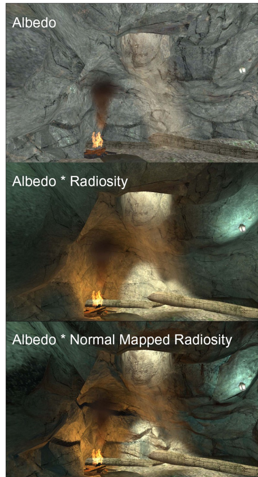
Figure 10: From top to bottom: Simple texturing (e.g. Ultima Underworld, Wolfenstein 3D, Doom I) - photos of a rock can be used for texturing the cave; Traditional lightmapping (e.g. Quake I) - combine the lightmap from the radiosity preprocessing step with the photo texture; Directional lightmapping (e.g. Half-Life 2) - three lightmaps and a normal map increase the scene detail significantly when combined with the photo texture. Image(s) taken from [McT04]; see section 4.5.
